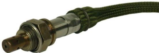
The Universal Exhaust Gas Oxygen (UEGO) sensor can measure a wide range of air/fuel mixtures. The sensor is based on ZrO<sub>2</sub> cells, held at an elevated temperature by an internal heater element. A current pumps oxygen between the sensing cavity and the exhaust to maintain a constant reference cell oxygen concentration. The measured value of this pumping current corresponds to the air/fuel ratio. Please request our installation datasheet for further details.
